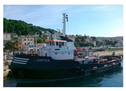
TUG boat multipurpose DSV (Diving Support Vessel) equipped with Surface AIR/Mixed Gas diving, optional support ROV, cable and flow line handling, hose loading and flushing systems. The vessel is designed to support Inspection, Repair, Maintenance and Construction in offshore operation s.
